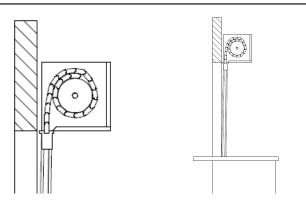
4. Holding the head case in its correct position, loosen the top screws from the guides and tilt to allow the door to be pulled down the guides. Push guides back into position and tighten screws.
