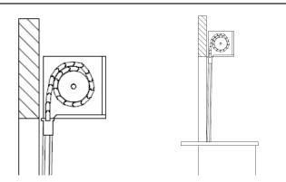
4. Holding the head case in its correct position, with the bottom rail out.
