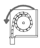
3. Pull the screen into installation position as shown above.
