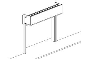
5 With the door pulled down in its closed position, the head case can now be fixed in place by screwing through the wings.
