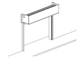
5 With the door pulled down in its closed position, the head case can now be fixed in place by screwing through the wings.
